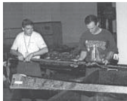
Figure 5. Application of braided sleeves to mandrels.
