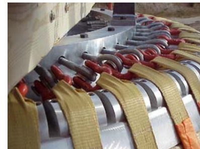
Figure 17. Vectran Belts Connection to Platen
