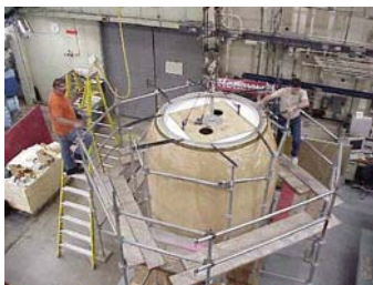
Figure 12. Restraint Layer: Mandrel with Runout Ring
