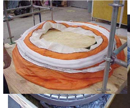
Figure 15. Slip Layer and Bladder Layer
