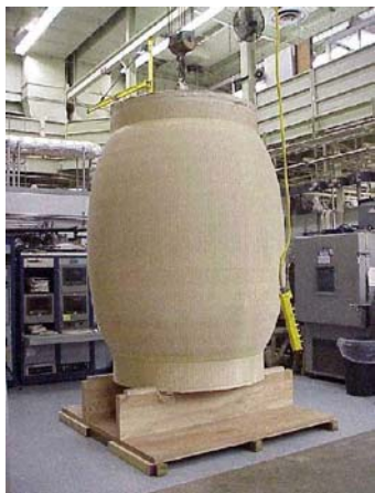
Figure 11. Full-Scale Restraint Layer with Mandrel
